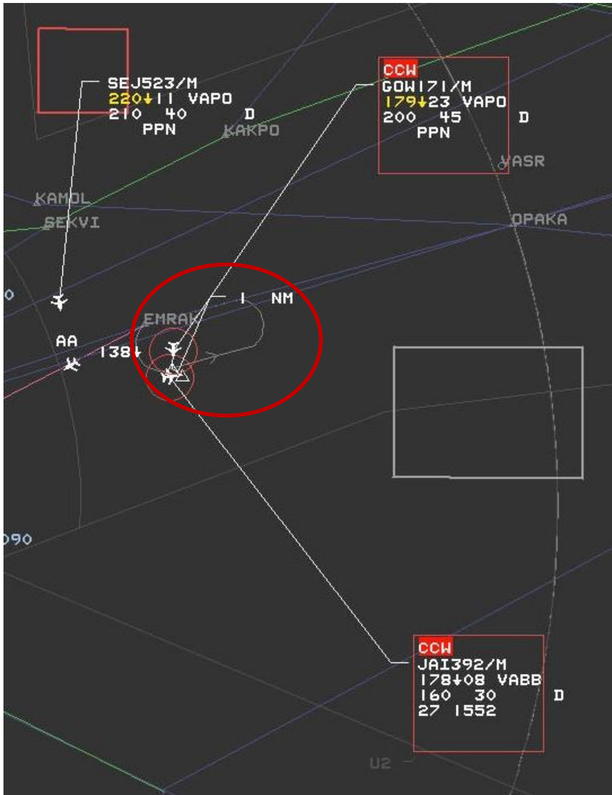
Figure 1: Airprox between GOW171 and JAI392 with vertical and lateral separation as 100 feet and 2.8 NM
